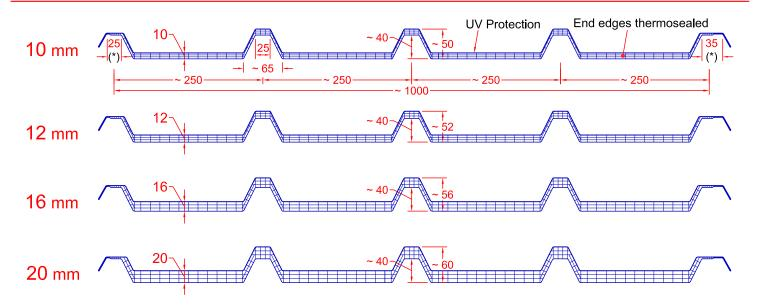
(\*) Standard width of lateral hooks 25 / 35 mm- alterable on request (min 20, max 40 mm)
